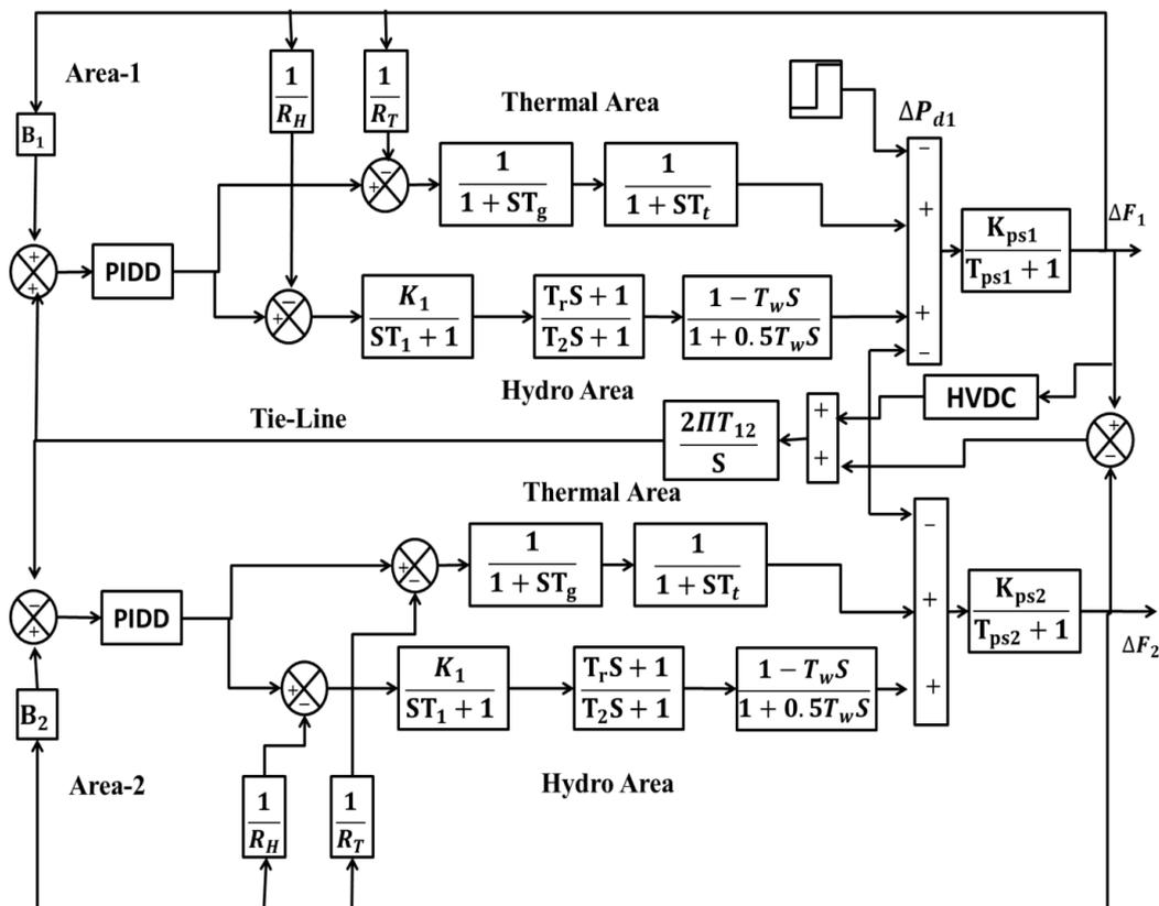
Figure 1: Model of DACTH system with HVDC tie-line.
