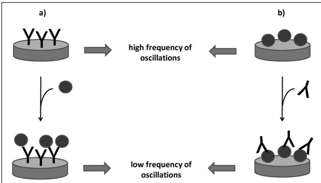
**Figure 2:** Piezoelectric Nano Biosensor for the detection of a) Antigen or b) Antibody. Piezoelectric crystals are represented as a blue color disc, Antigens are represented as red color balls, and Antibodies are represented as Y due to the appearance of immunoglobulin's [13]
