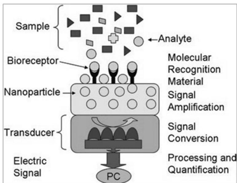
**Figure 1:** showing the components of the Biosensor along with its function. Blue color balls are the analytes, yellow color balls are Nanoparticles, and Y-shaped black color receptors are Bioreceptors [14].
