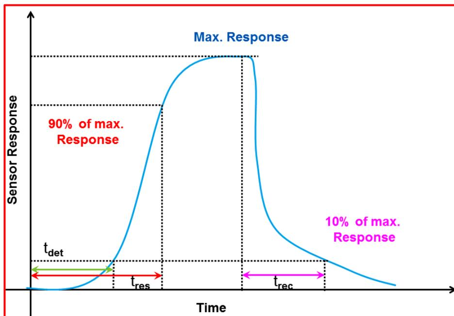
Figure 6: response, recovery and detection time.
