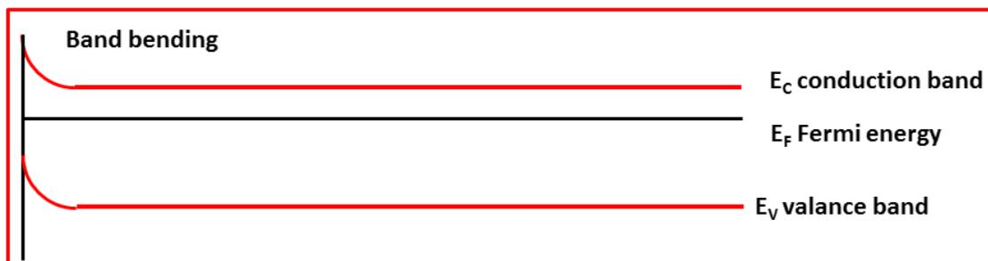
Figure 4: Energy band diagram of MOX (n-type) on oxygen chemisorption.
