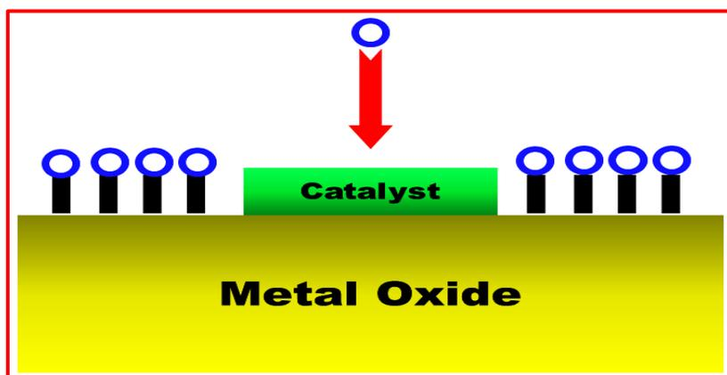
Figure 8: Schematic of spill over phenomena.
