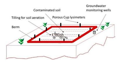
Contamination deeper than 1.7 metre are excavated and transported to fresh lands for bioremediation. They are then spread in thin layers and repeatedly tilled to ensure uniform aeration. The base is kept impermeable to minimize leaching of pollutants and nutrients. Nutrients and moisture are added to help the autochthonous germs in degrading the waste. The energy cost is negligible here but vast land area is required.
