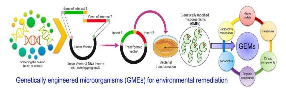
Microbes have genetic material that encodes enzymes for breaking down of waste. Exposure to contaminants lead to acquisition of appropriate metabolic machinery. The indigenous microflora on polluted sites may lack certain desirable traits required for effective bioremediation. These traits can be incorporated into bacteria using molecular biology tools of gene cloning and insertion. These genetically modified microbes or GEMs can be used for
