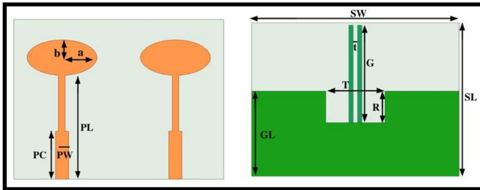
**Figure 1: Simulated MIMO antenna (a) front, and (b) back view**
