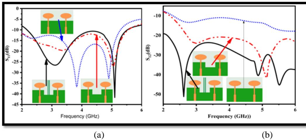
**Figure3: Evolution steps of (a) Reflection coefficient ( $S_{11}$ ), (b) Transmission coefficient ( $S_{12}$ )**
