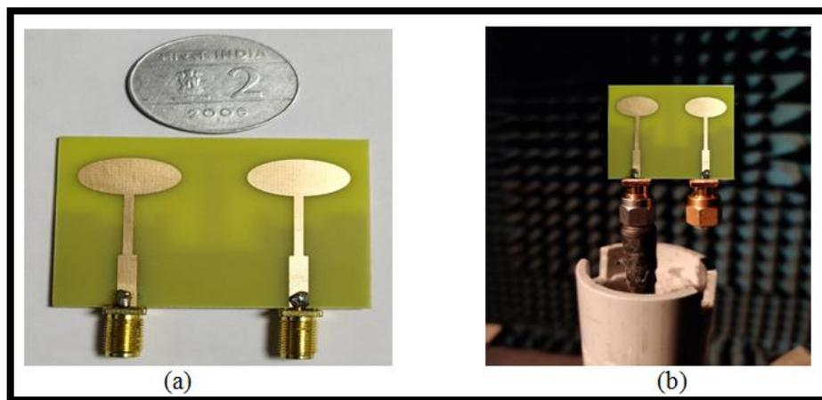
**Figure 2: Fabricated (a) MIMO antenna, and (b) experimental setup**
