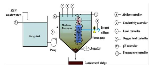
**4. Bio Augmented Activated Sludge Process:** An activated sludge system based on bioaugmentation with specialized microorganisms can be a powerful tool to enhance the efficiency of a wastewater-treatment process through improved flocculation and settling of activated sludge.
