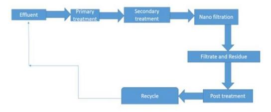
NF membrane is mostly preferable method due to no need of any chemical in functioning, heavy metal and organic reduction, removal of multivalent ions, less amount of waste discharge, less operational cost. Pore radius, Thickness-Porosity ratio and Charge density of the membranes are important specifications in removal process.
