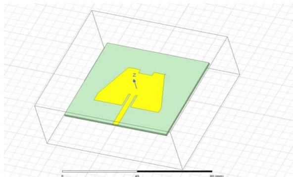
**Figure 1:** M shape substrate patch antenna
