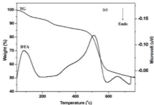
Figure 1: TG and DTA curves of  $[\text{Pr}(\text{N}_2\text{H}_4)(1-\text{C}_{10}\text{H}_7\text{COO})_3]\cdot 2\text{H}_2\text{O}$  compound
