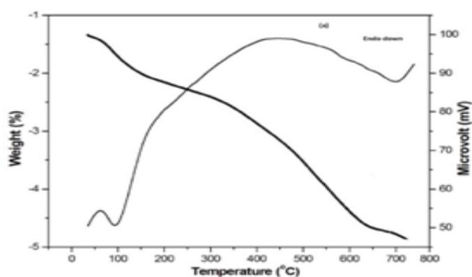
Figure 3: TG and DTA curves of curves of  $[\text{Pr}(\text{N}_2\text{H}_4)_2\{\text{C}_{10}\text{H}_6(1-\text{O})(2-\text{COO})\}_{1.5}]\cdot 3\text{H}_2\text{O}$  compound
