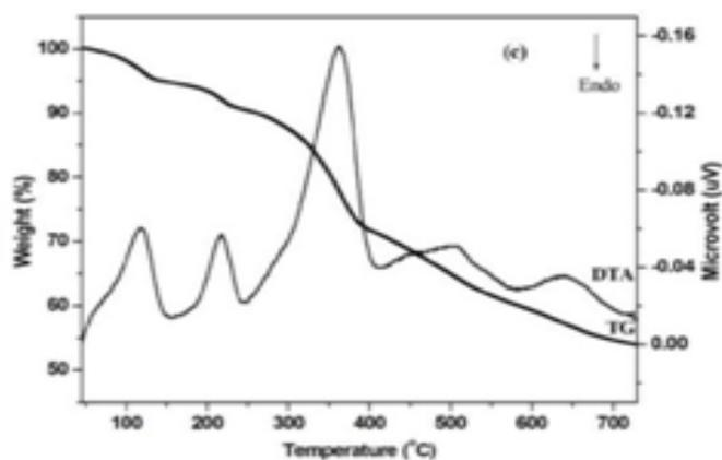
Figure 2: TG and DTA curves of  $[\text{Pr}(\text{N}_2\text{H}_4)_2(2-\text{C}_{10}\text{H}_7\text{COO})_3]\cdot 2\text{H}_2\text{O}$  compound
