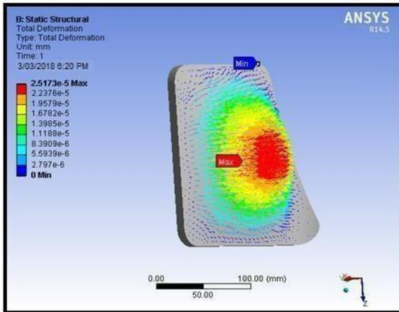
**Figure 5:** Deformation in Glass Material
