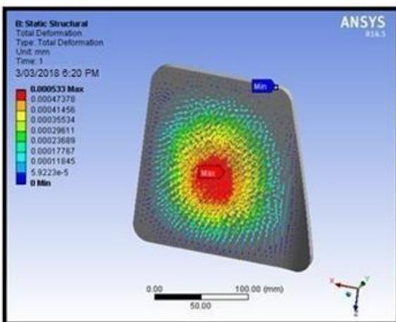
**Figure 9:** Deformation in Poly Vinyl Butyl material(PVB)
