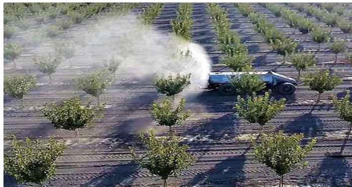
Figure 3: Autonomous spraying system for orchards
