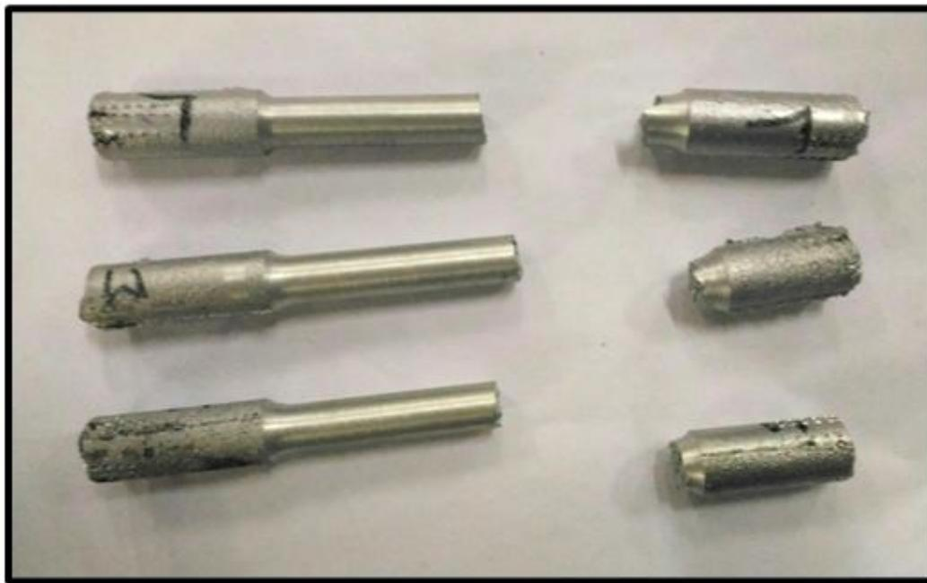
**Figure 9:** Fractured Specimen after Tensile Test.
