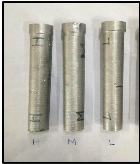
**Figure 4:** Test Specimens (Showing Track Distance of all 3 specimens)
