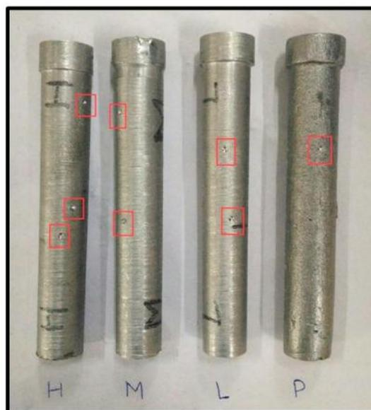
**Figure 6:** Specimen Showing Indentations
