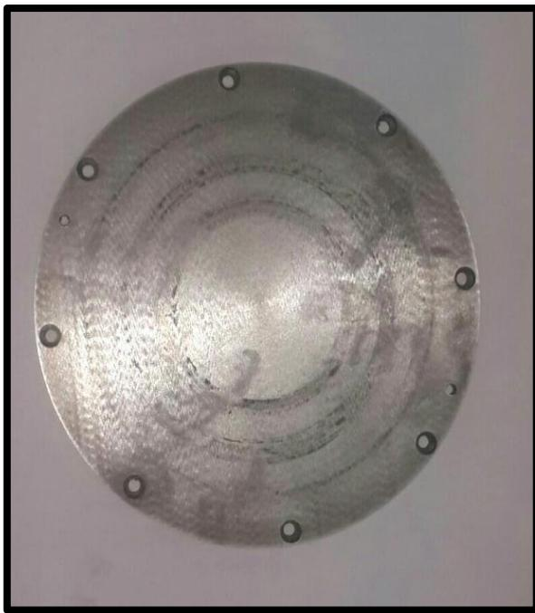
**Figure 3:** Wear on disc after test
