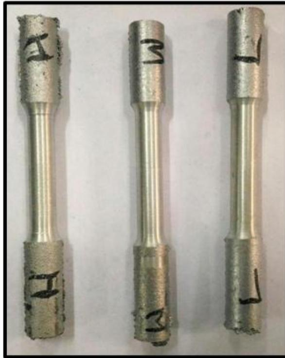
**Figure 7:** The Specimens Prior Tensile Test.
