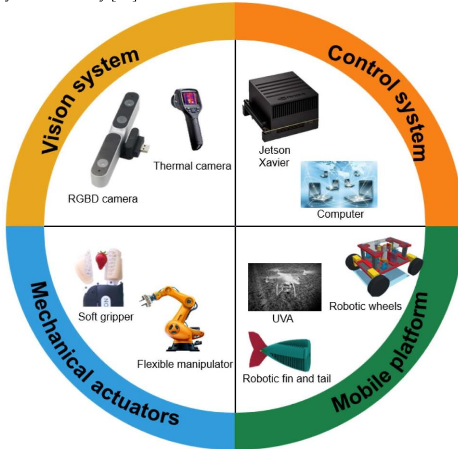
Figure 9: Components of advanced agricultural robots [76, 77].
