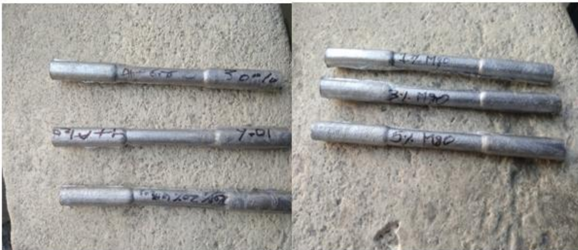
Figure 4.5: Specimen before tensile test.
