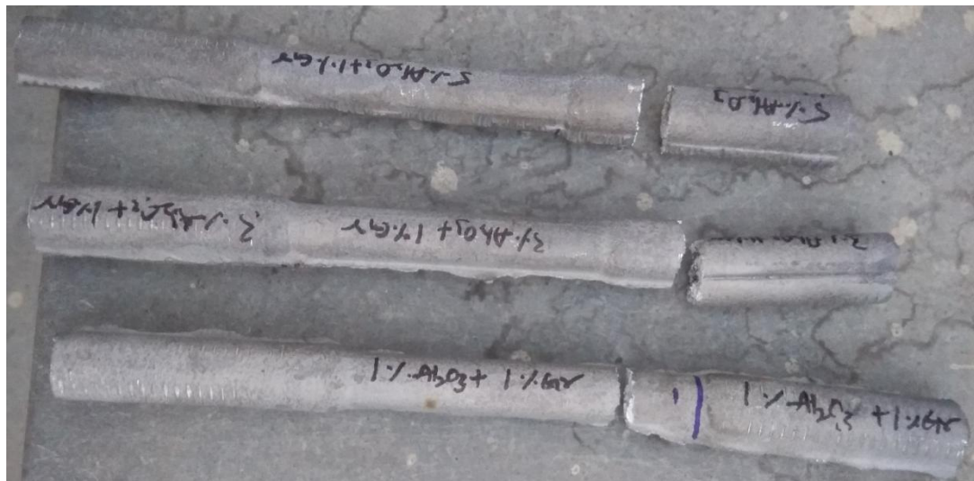
Figure 4.7: Actual samples of LM 25 + 1%, 3% and 5% \text{Al}_2\text{O}_3 + 1% Gr after tensile test
