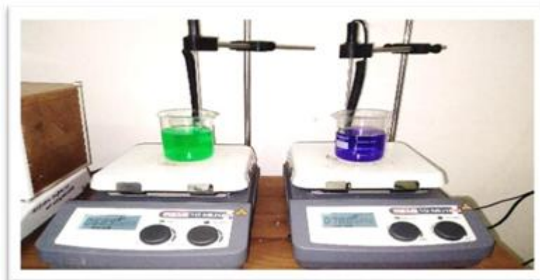
Figure 1: NiP (left) and NiB (right) coating solution bath
