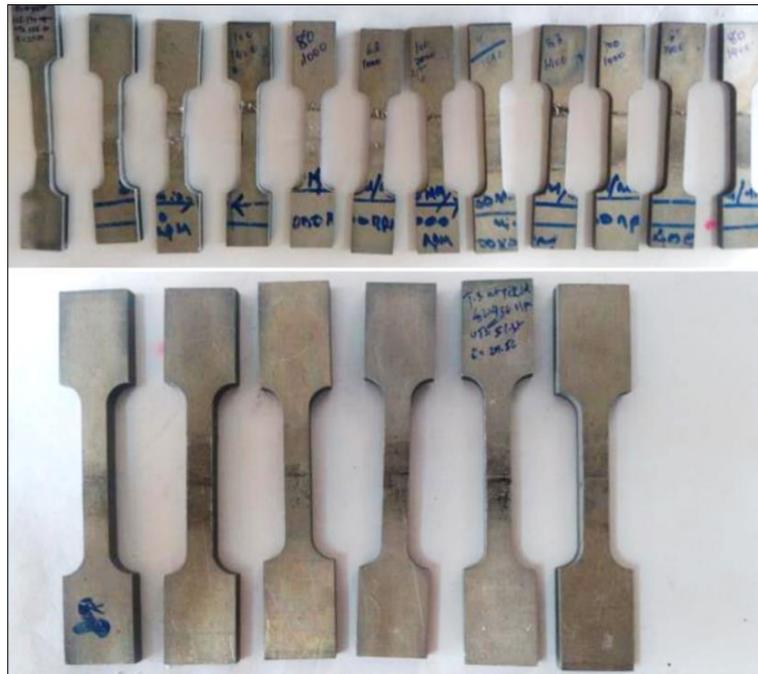
**Figure 1:** Tensile Test specimens.
