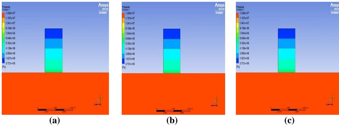
**Figure 4:** Pressure contour of the rectangular crack of  $0.5 \times 10^{-6} \text{ m}^2$  at (a) 70 bar inlet pressure, (b) 80 bar inlet pressure, (c) 90 bar inlet pressure
