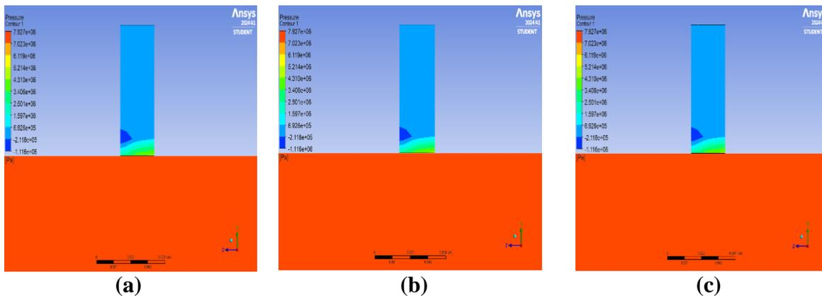
**Figure 8:** Pressure contour image of the circular crack of area  $12.56 \times 10^{-6} \text{ m}^2$  at (a) 70 bar inlet pressure, (b) 80 bar inlet pressure, (c) 90 bar inlet pressure
