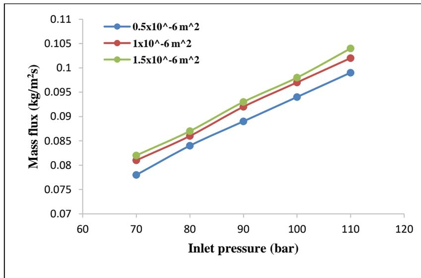
Figure 3: Variation of maximum mass flux with Pressure for rectangular cracks
