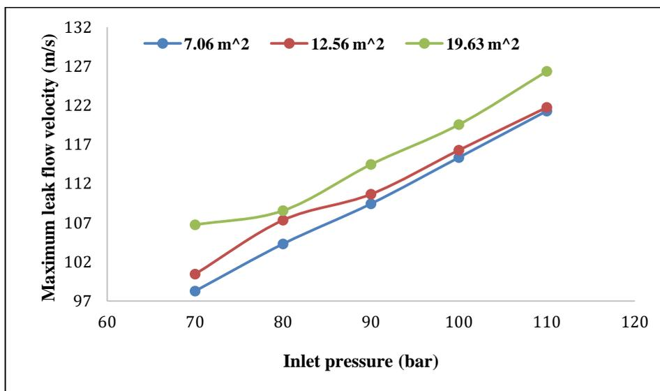
**Figure 6:** Maximum leak flow velocity vs. Pressure graph for circular cracks
