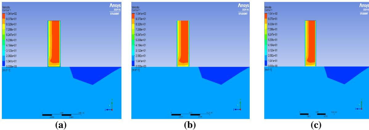
**Figure 9:** Velocity contour image of the circular crack of area  $12.56 \times 10^{-6} \text{ m}^2$  at (a) 70 bar inlet pressure, (b) 80 bar inlet pressure, (c) 90 bar inlet pressure
