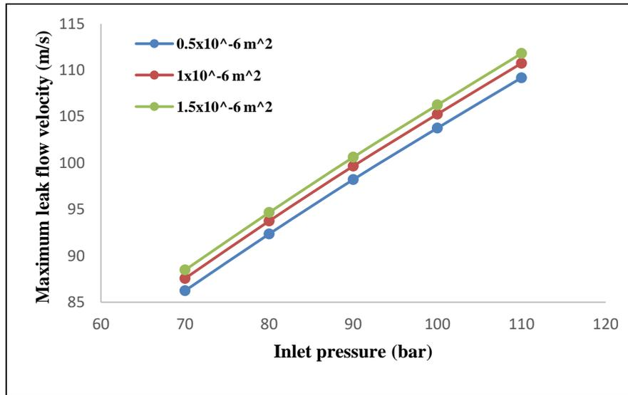
Figure 2: Variation of maximum leak flow velocity with pressure for rectangular cracks
