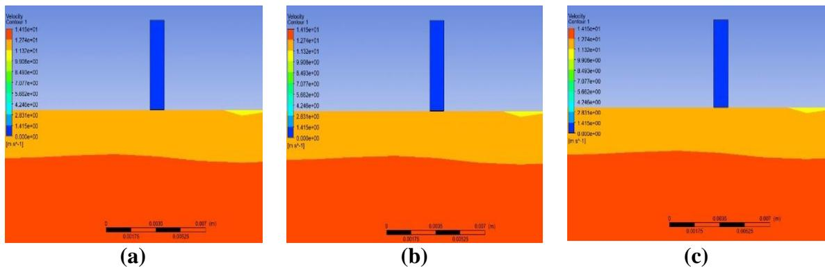
**Figure 5:** Velocity contour of the rectangular crack of area  $1.5 \times 10^{-6} \text{ m}^2$  at (a) 70 bar inlet pressure, (b) 80 bar inlet pressure, (c) 90 bar inlet pressure
