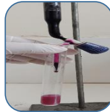
H - Estimation of percent dissolution of calcium oxalate by titrimetric.
