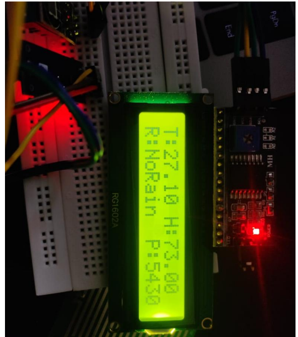
3. LCD Displaying Real time data
