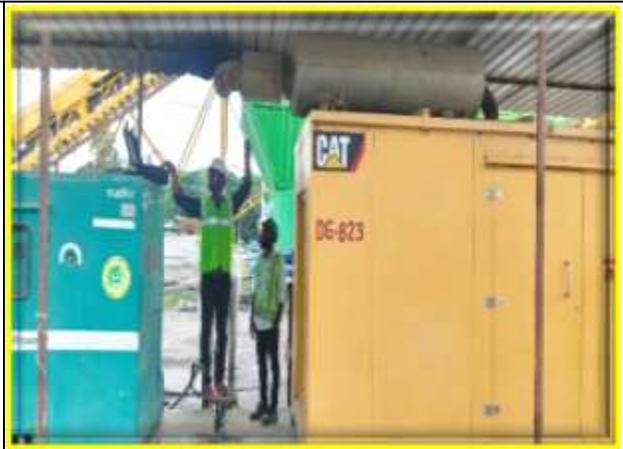
**DG Stack Emission and DG Noise Sample Collected @ Chainage Number 18 + 500 Km Camp Site.**
