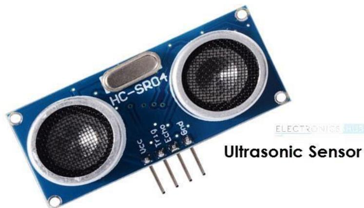
Using the time of flight of the sound wave, an Ultrasonic Sensor can measure the distance of the object (similar to SONAR). The Doppler Shift property of the sound wave is used to measure the velocity of an programming with hardware controllers
