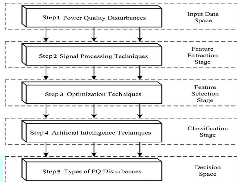
Fig 2: Block diagram of PQ Disturbances Detection and Classification System
