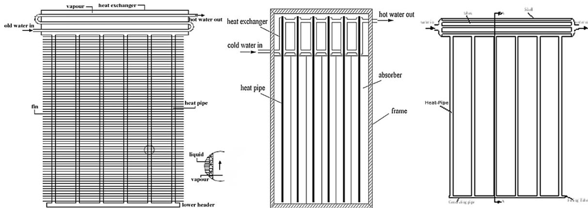
**Figure: 7 Different Condenser Arrangement in Solar Collector**
