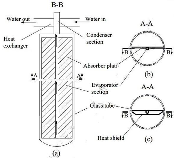
**Figure: 5 Heat Shielded ETC**
