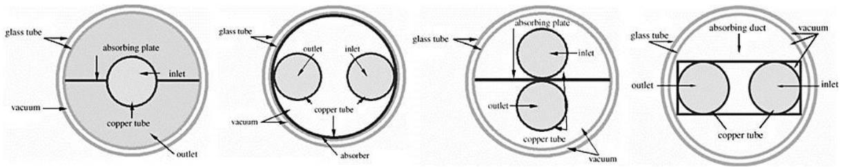
**Figure: 4 Differences in collector Centre Distance in ETC**
