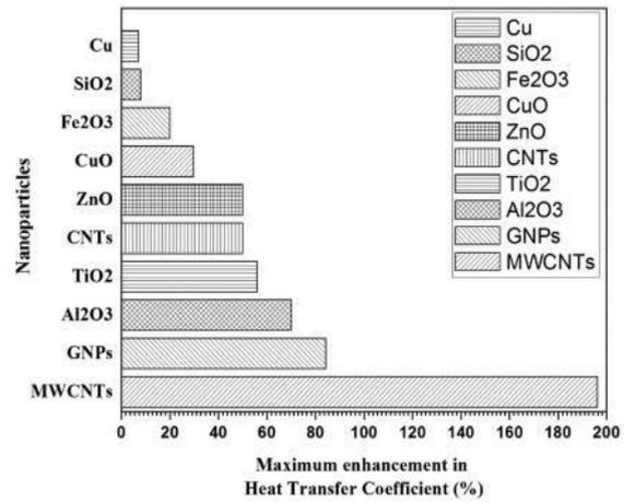
Figure: 17 Maximum Enhancement in heat transfer coefficient (%)
