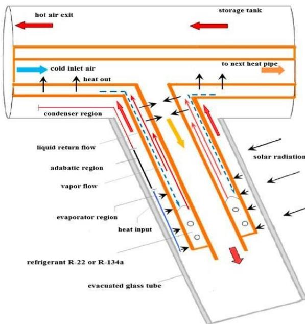
**Figure: 12 Double Concentric pipe ETC**
