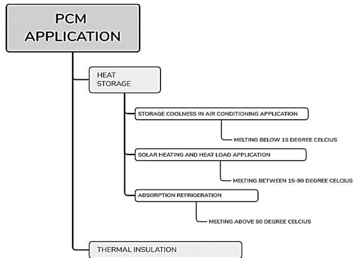
**Figure: 22 Different PCM Application**
