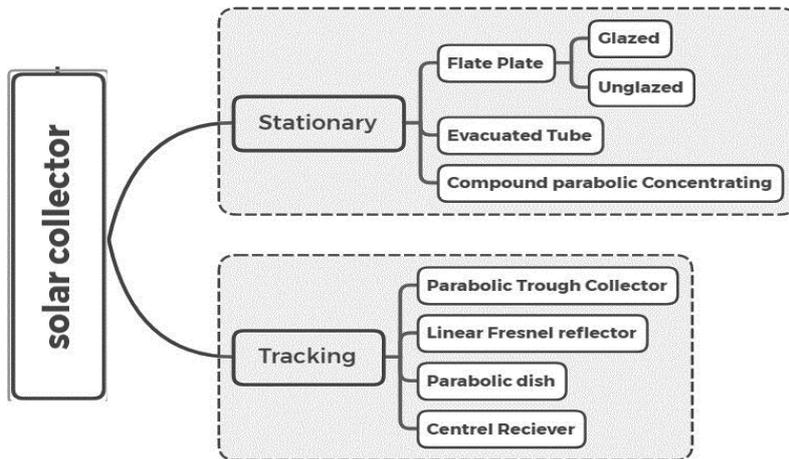
**Figure: 3 Classification of Solar Collector**
