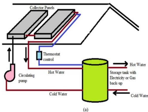
Figure: 1 Passive solar water heating system with indirect circulation (PSHWS)
