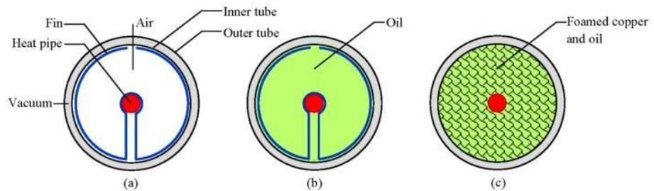
**Figure: 11 ETC Filling with (a) Air (b) Oil (c) Copper Foam**
