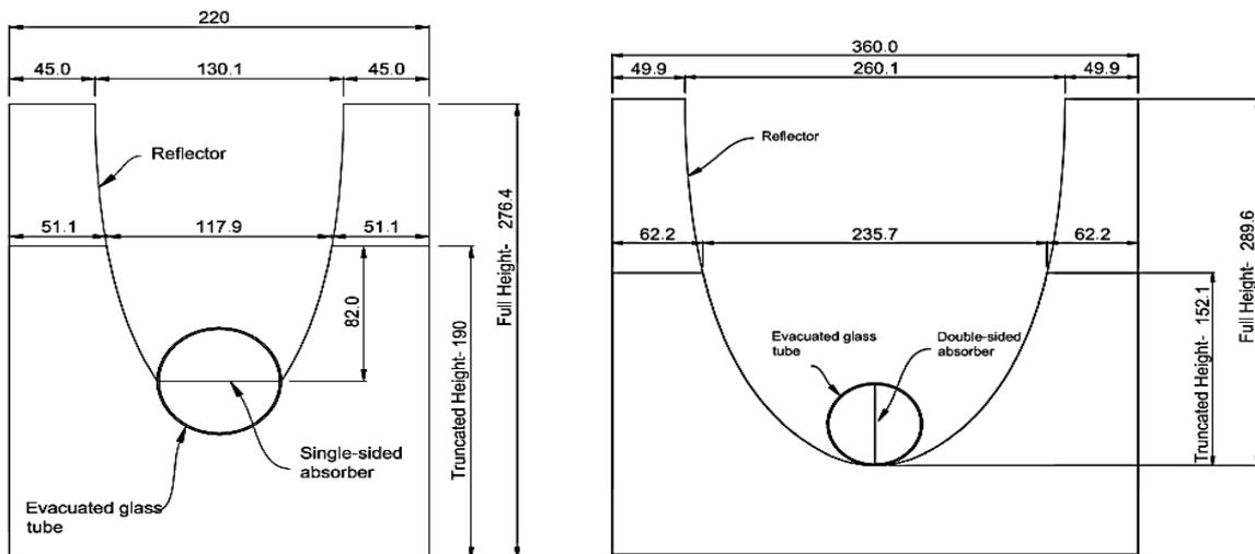
**Figure: 6 Side Section View of the Full and Truncated SSACPC & DSACPC Solar Collector**
