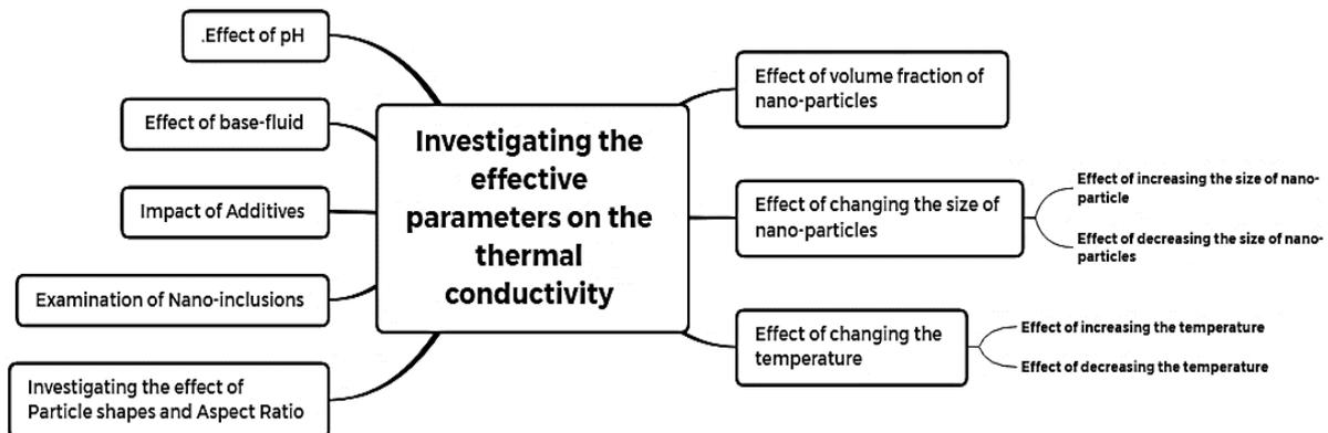
Figure: 15 Effective Parameter on Thermal Conductivity of Working Fluid
