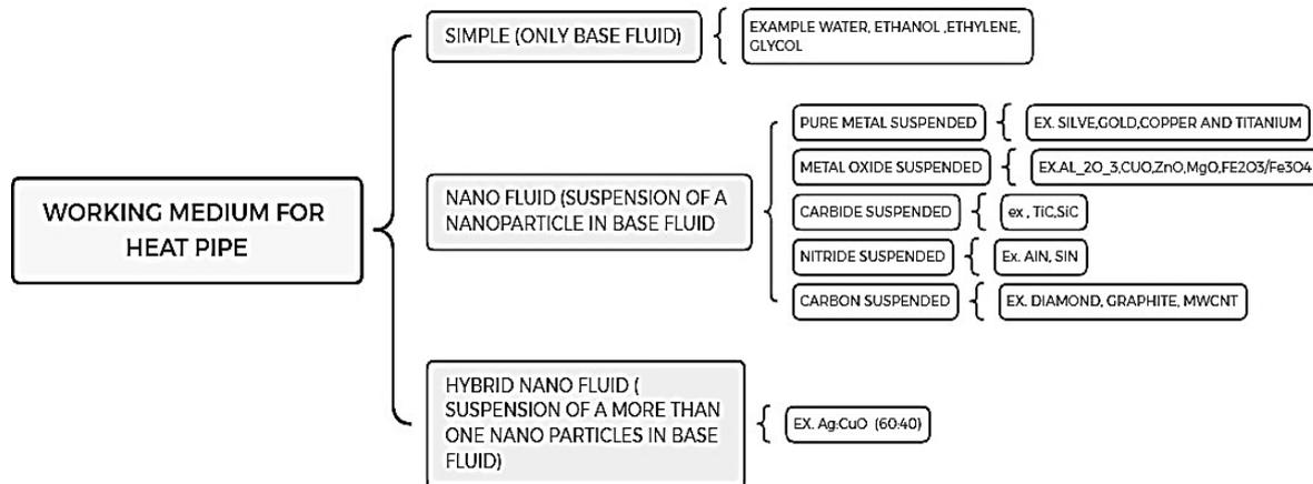
Figure: 14 Working Fluids for Heat pipe
