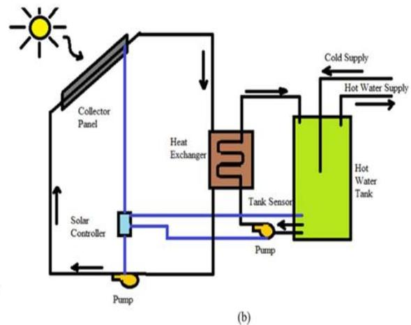
Figure: 2 Active solar water heating system with direct circulation (ASHWS)
