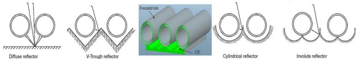
**Figure: 13 Different types of concentrator**
