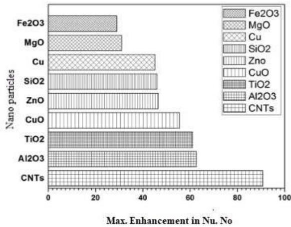
Figure: 16 Max. Enhancement in Nu no for Different Nanoparticles
